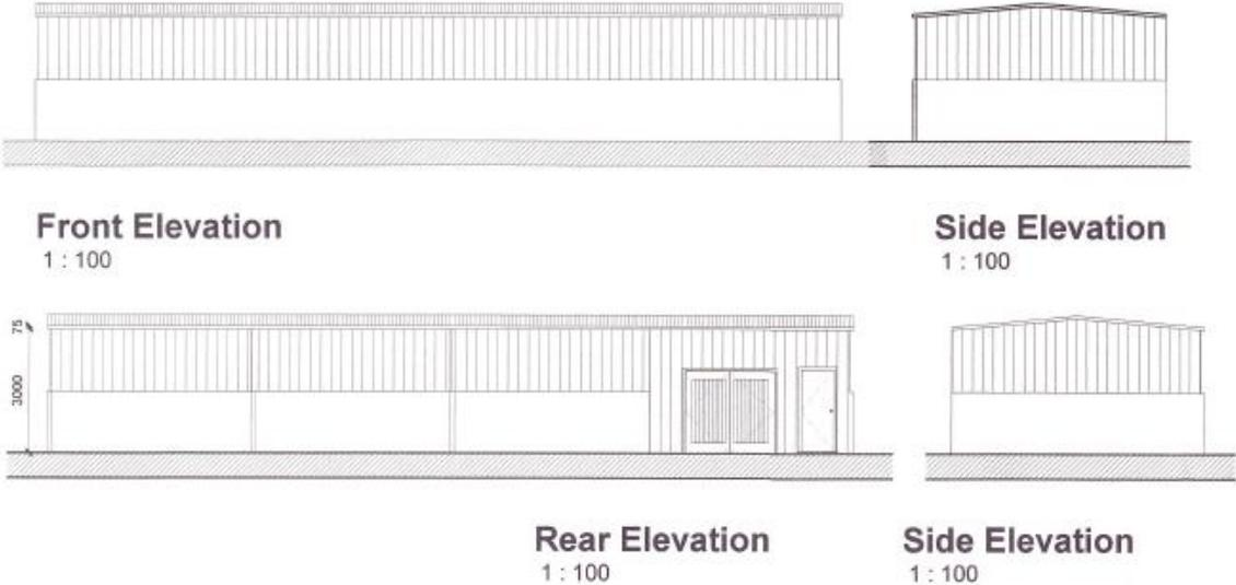
**Fig 3: SHED 1 - Elevations**
