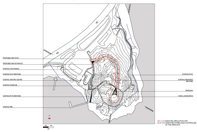
Fig. 5: Site plan as proposed.
