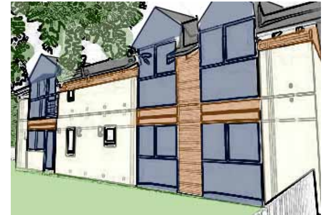
Passive Solar Gain; proposed orientation allows maximum solar access to the facades with living spaces
