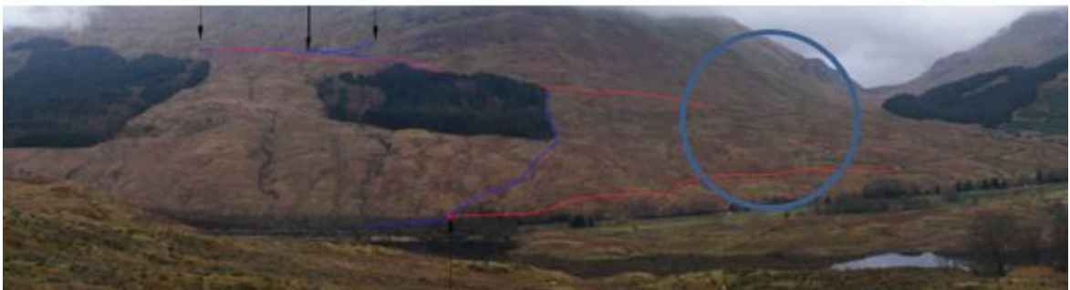
Figure 8: View of proposed scheme looking south from Breadalbane - Schiehallion Wild Land Area. Blue circle= Existing track into Benmore Glen. Red lines= Proposed access tracks. Blue line = Buried pipeline. Arrows point towards the location of the intake structures.
