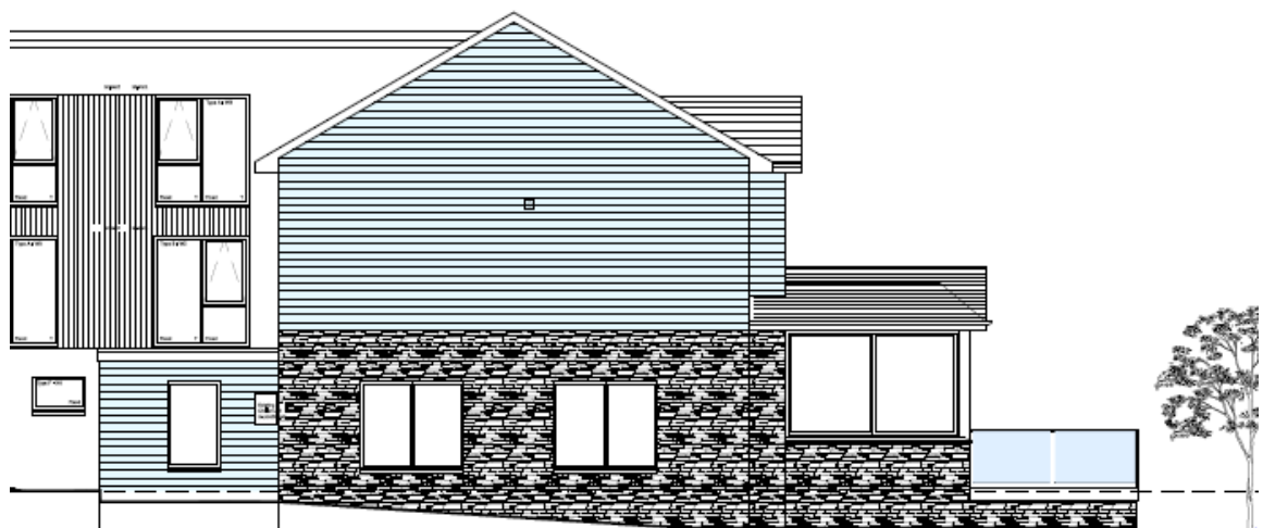
West Elevation as Proposed showing front extension and rear extension, glass balustrade and new cladding to first floor.
