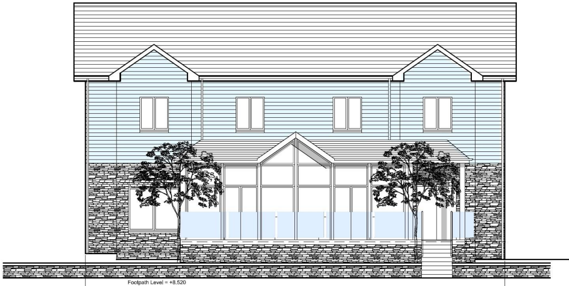
South (Roadside) Elevation as Proposed showing front extension, glass balustrade and new cladding to first floor.
