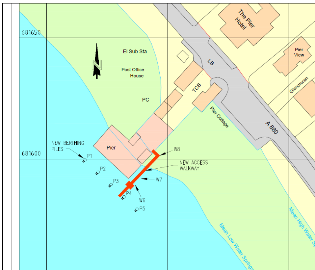
Figure 1: Site plan which shows the location of the proposed structures and identifies Mean High Water springs and Mean Low Water Springs.
