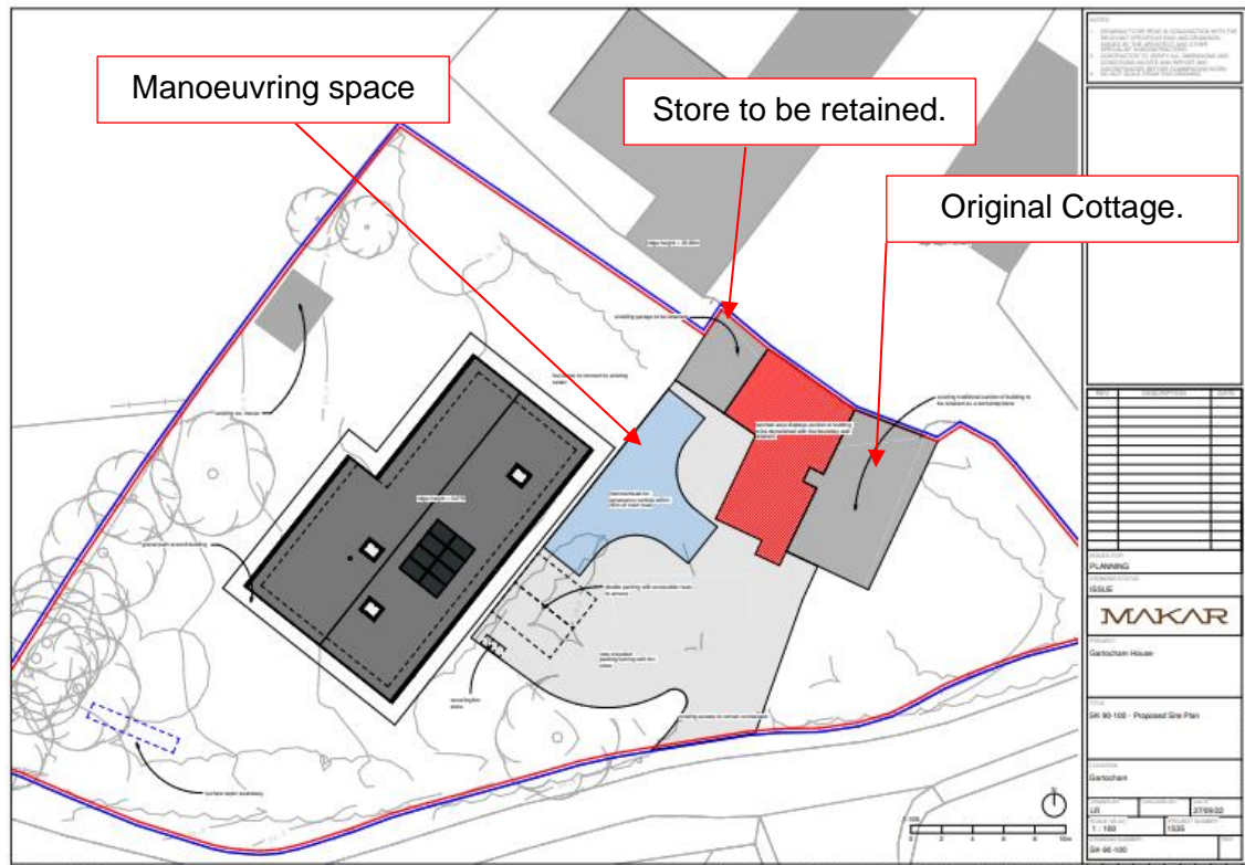
Figure 8: Proposed site layout plan showing location of replacement dwelling and parking arrangements and the existing cottage and store (grey) highlighting the flat-roofed part to be demolished (red).
