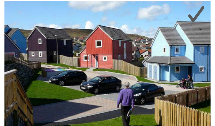
Good example of coralled parking freeing up building fronts (c. Richard Gibson Architects)
