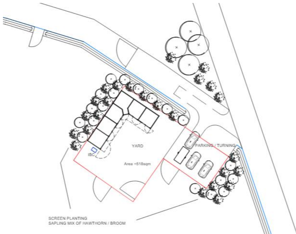
Figure 8: Proposed Site Plan showing Stable Building, Parking Area and Proposed Planting along boundaries
