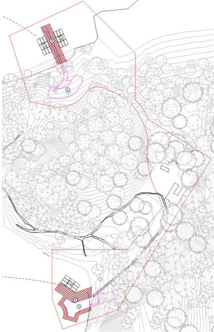
Figure 12: Site Plan of Proposed Temporary Construction Pontoons - showing the proposed pontoons to be utilised during construction for distribution and handling of materials and to be removed upon completion of development.
