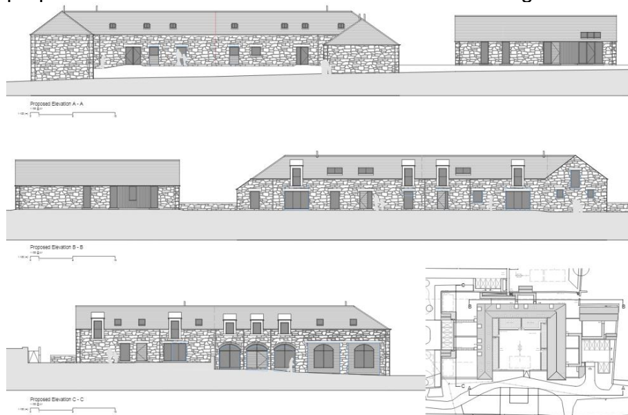
Figure 9: Proposed Elevations – plan submitted showing the proposed finished appearance of the steading and adjacent single dwelling.
