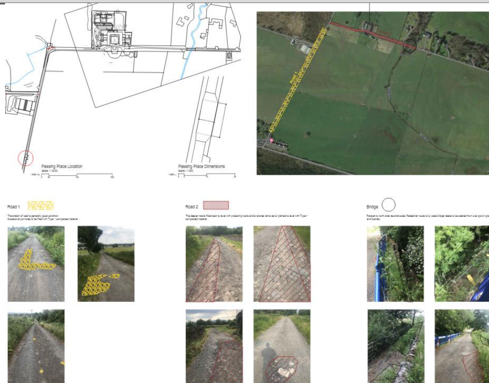
Figure 12: Proposed Road Repairs – plan submitted detailing the location and proposals for passing place, road and bridge repairs along Coldarach Road (outlined in yellow) and Coldarach Lane (outlined in red).
