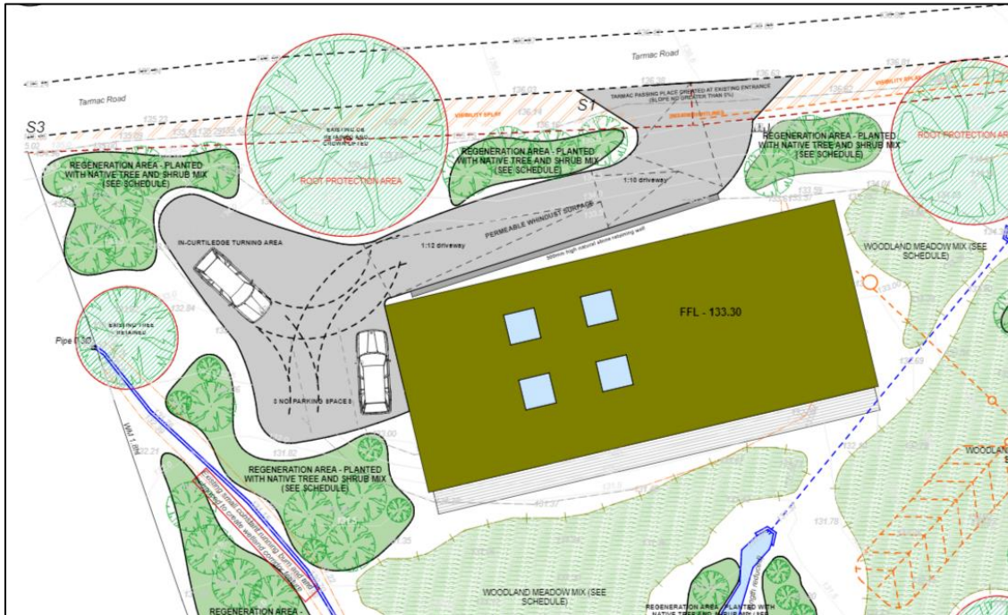
Figure 4. Site Plan – Site Plan showing the proposed access arrangements from Glen Road: tarmac passing place created at entrance, permeable whindust surface driveway, in-curtilage turning area, 3No. parking spaces.
