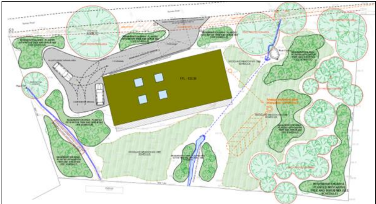
Figure 8. Proposed Planting – Plan showing the proposed landscaping and planting across the site including areas of native tree and shrub mix and woodland meadow mix.
